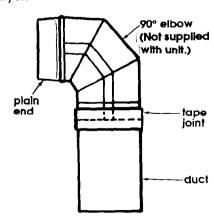
**5.** Attach a three- or four-section elbow to the straight duct using duct tape. Repeat with the other elbow and straight duct.
